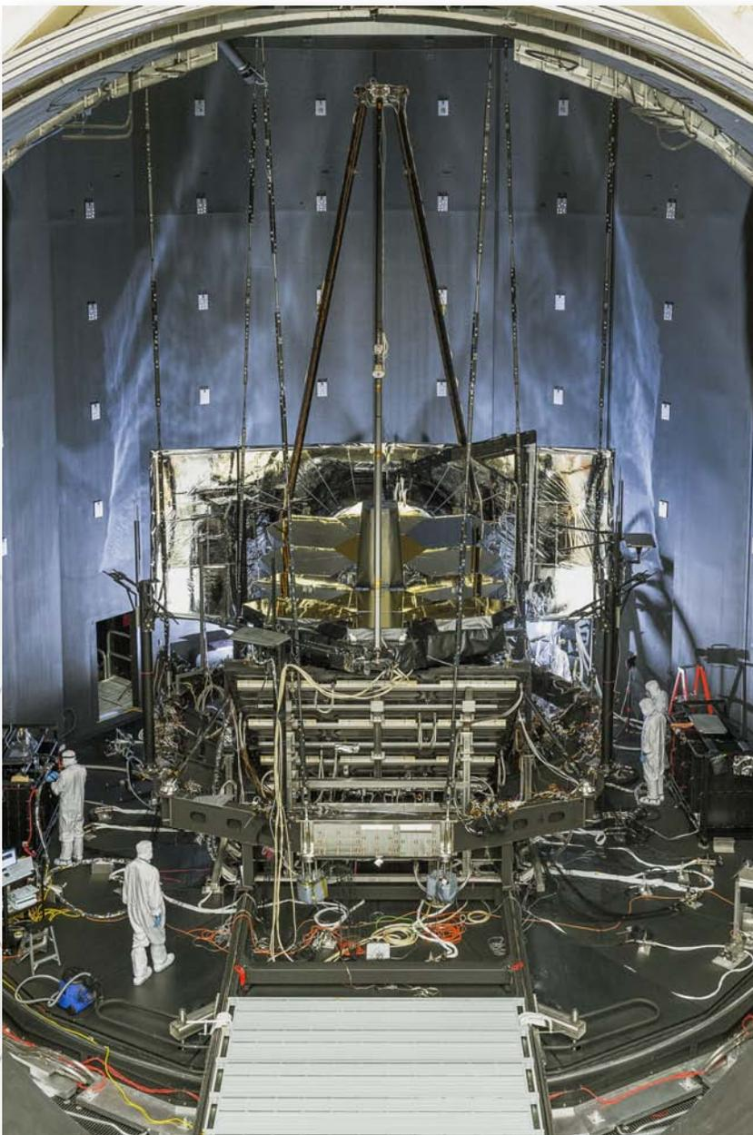
*Figure 3. The Pathfinder structure, thermally configured for the Thermal Pathfinder Test to be carried out shortly at the Johnson Space Center. The dummy Aft Optical System (AOS) is visible in the center of the primary mirror segments. Among those segments can be seen one gold-coated flight-spare beryllium segment (just in front of the AOS), one uncoated beryllium engineering unit segment, and ten gold-coated aluminum thermal simulator segments.*
